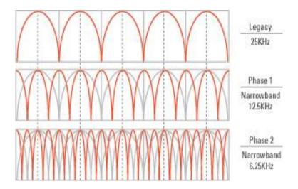
The FCC expects land mobile licensees to ultimately transition to equipment that supports a 6.25 kHz channel bandwidth (or less). The FCC mandated that all equipment for the 700 Mhz public safety band use 6.25 kHz channels or less on January 1, 2015.
